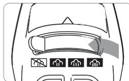
Before filling, slide the steam selector to off (☒). **Make sure the iron is unplugged.**
