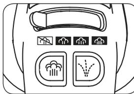
**Steam Selector:** Slide the steam selector to set the amount of continuous steam. The iron can only produce steam when the fabric selector knob is set to the wool (●●), cotton, or linen range (●●●). Allow the iron to heat up (solid green status light) before activating the steam control. Steam will be produced as soon as the iron is lowered. Steam will stop when iron lifts up.
